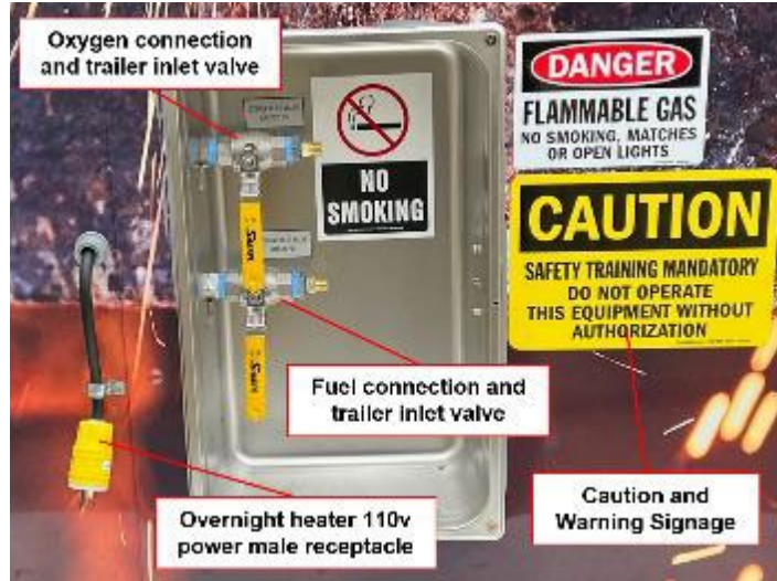
Oxygen and Fuel Supply Connections (Trailer Side)
